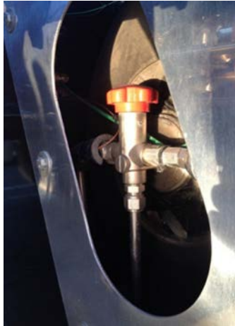
Figure 49 The cylinder valve handle on side mount systems should be at the 12 o'clock position as shown above.
