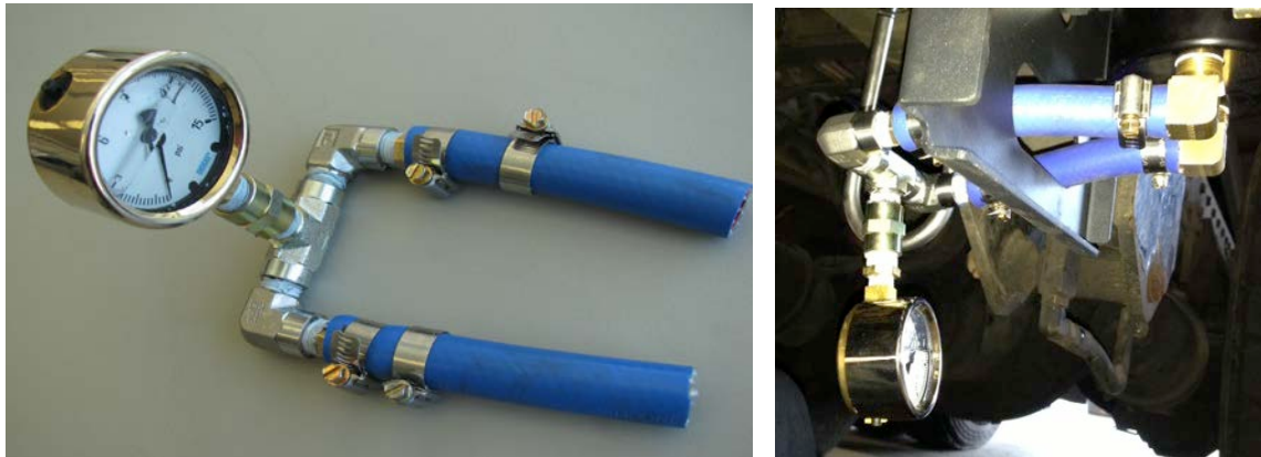
Figure 69 A shop-built regulator test jig.
