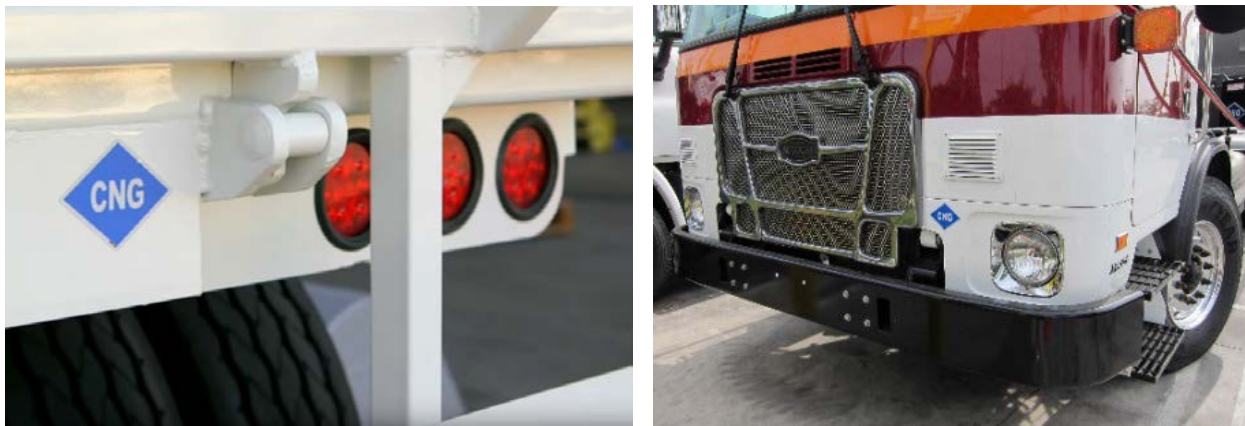
Figure 9 Left: CNG fueled vehicles are identified by a blue and white decal on the right rear of the vehicle. Right: A CNG decal may also be located on the front of the vehicle as shown.
