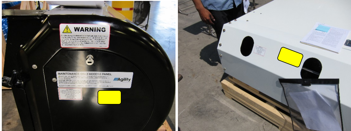
Figure 17 PRD vent line decal locations shown in yellow.
