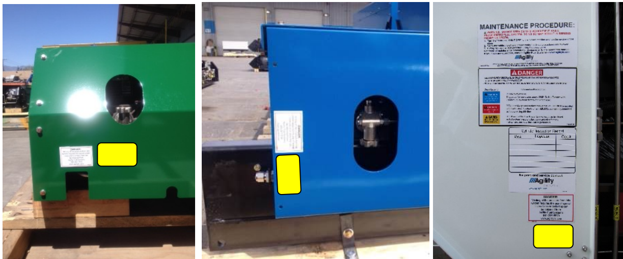
Figure 18 More PRD vent line decal locations, shown in yellow.
