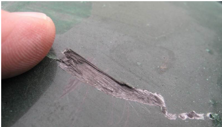
Figure 29 Damage from impact can be seen as missing composite sections.
