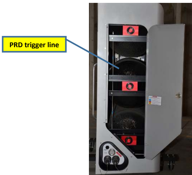
Figure 24 Back of cab system showing area PRD trigger lines behind the side door. Similar trigger lines are routed on the opposite side.
