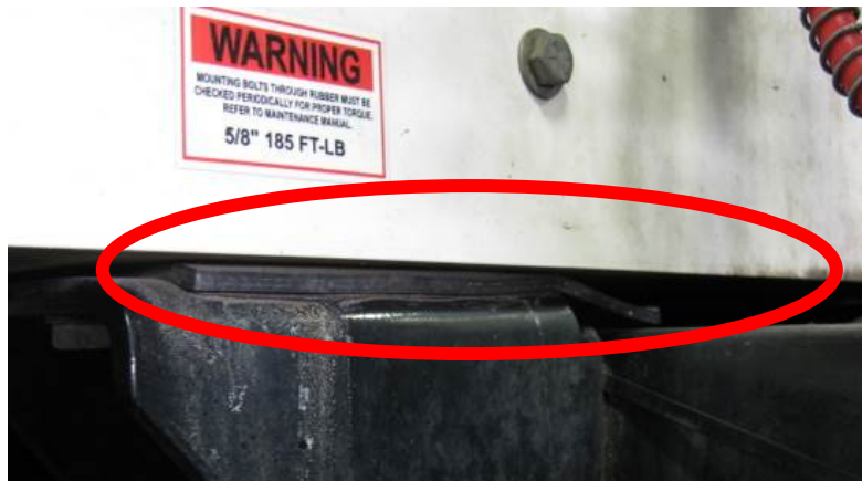
Figure 38 Rubber isolator between the BTC cabinet and vehicle chassis on a four year old system with 316,000-plus miles. A quick look indicates the rubber pad is in good condition.
