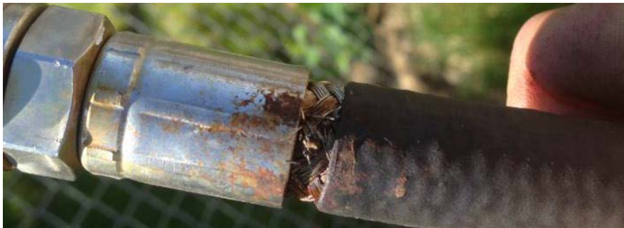
Figure 34 Corrosion on CNG hose braid and fitting.
