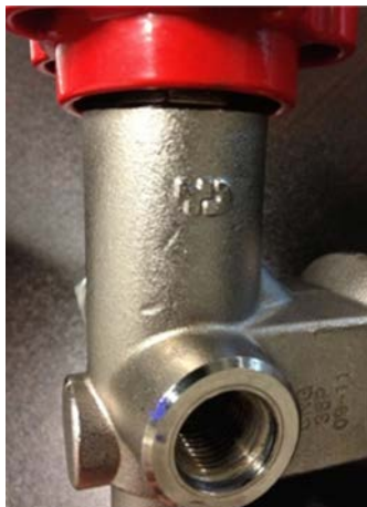
Figure 52 This type of manual cylinder valve is prone to fail in the closed position.
