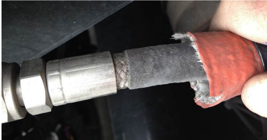
Figure 33 If the hose is covered with a sleeve, move it to enable inspection of the braid and ferrule. Remember to inspect the sleeve for damage, too.
