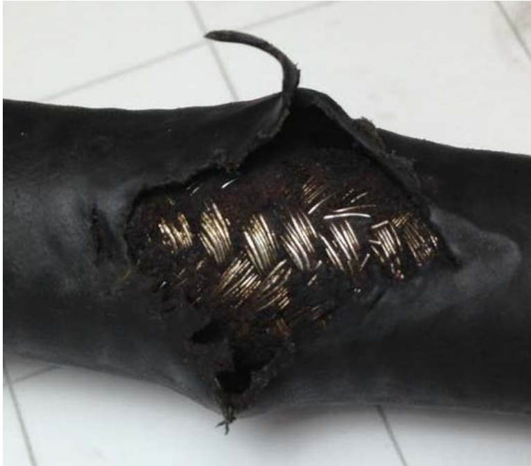
Figure 36 The outer covering of this hose has been worn away due to abrasion. It should be replaced and secured properly away from any other surfaces or components.
