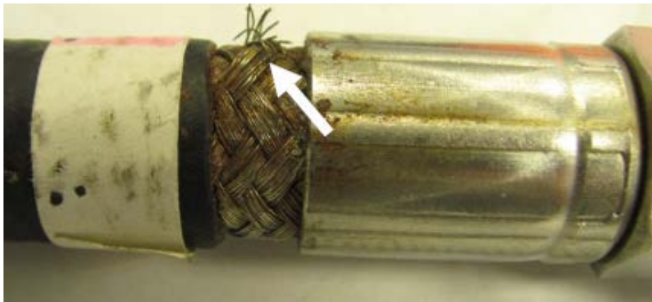
Figure 35 Broken wire strands in the braid are also evidence of compromised hoses.
