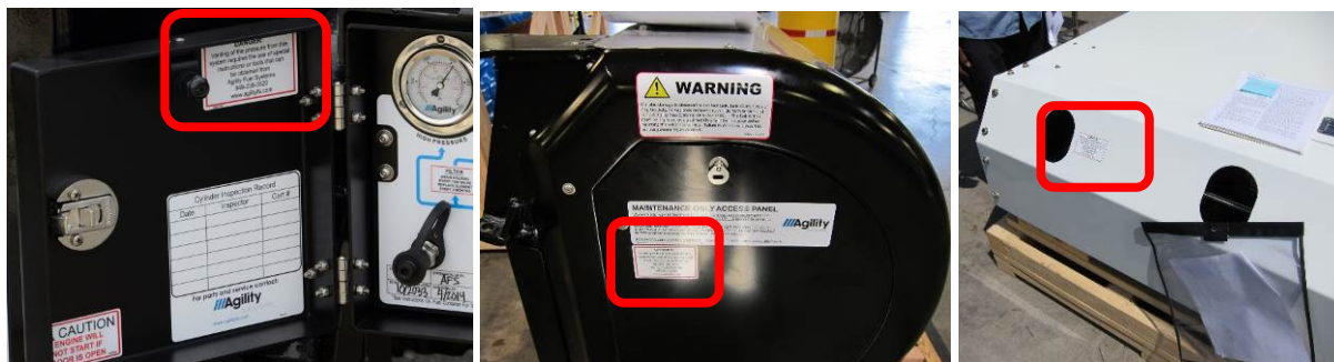
Figure 15 The “Danger venting gas” decal is placed in several locations, usually near cylinder and bleed valves.
