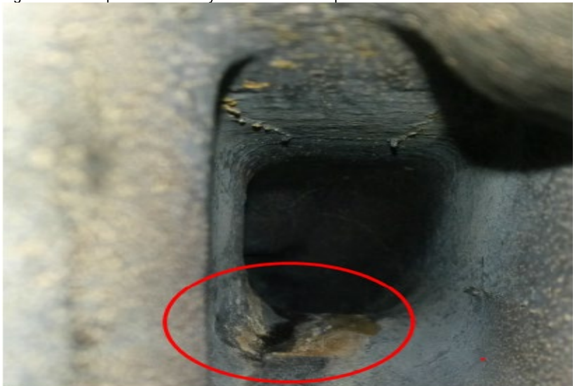
Figure 4 – example of cracked cylinder head intake port.
