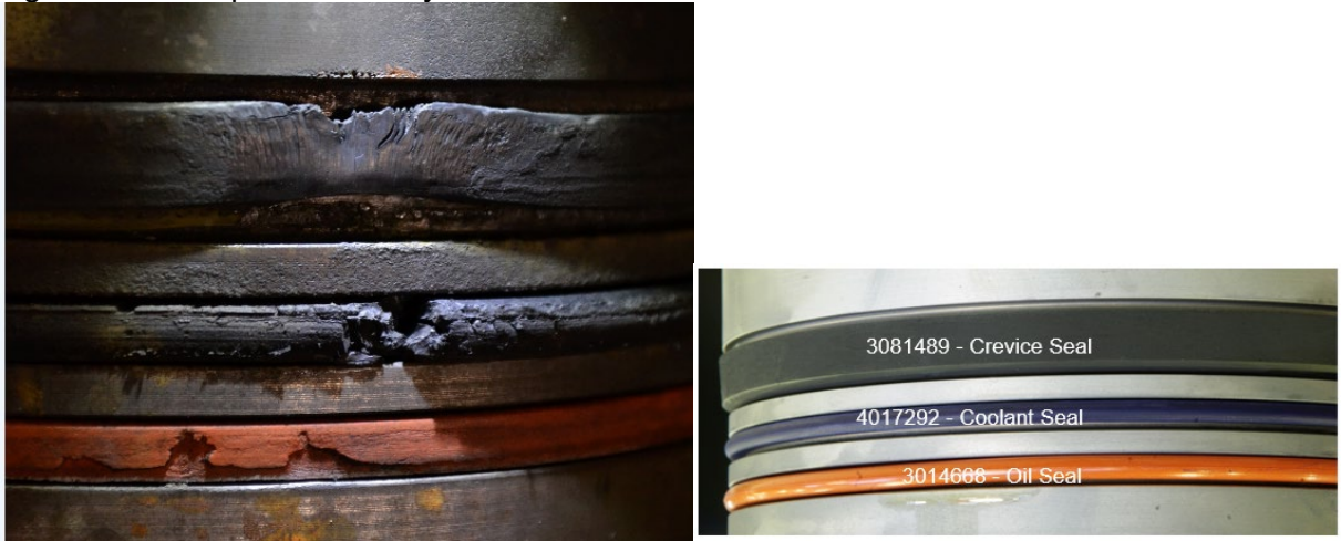
Figure 5 – example of failed cylinder liner seals vs new for reference
