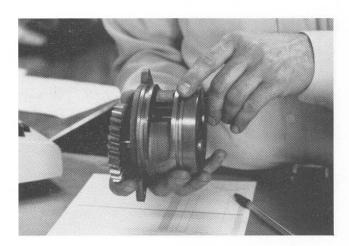
63. Also, there are two different size "O" rings for mounting the lube pump. The larger "O" ring is installed on the front of the lube pump, and the smaller one on the back. Be sure to tell your customers that if the "O" rings are properly installed, the pump will go into place easily, but if they have to use force, the "O" rings are in the wrong position.
