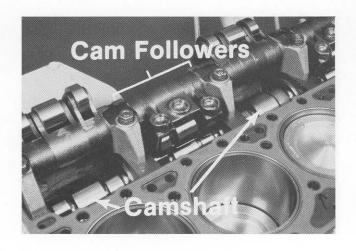
42. The high location of the camshaft allows the use of short push rods resulting in a stiffer overhead valve and injector train for more precise control.
