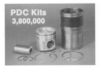
55. Most of the replacement parts for the L-10 are structured in complete kits with all of the necessary gaskets and mounting hardware included. For easy recognition, you'll find that the new PDC Structured Service Kits for the L-10 and our other engines are identified with a 3,800,000 series part number.
