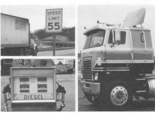
16. The soaring cost of diesel fuel has forced the trucking industry to concentrate heavily on fuel economy. Lower speed limits, air shields, radial tires, thermatic fans, and aerodynamically designed cabs and trailers have all been major factors in reducing horsepower requirements. Together, these changes have created a widespread need for a smaller, extremely efficient, heavy-duty, high performance engine.
