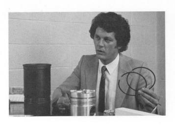
61. Here's another example...These intermediate rings are used on your high-powered engines to work along with the top compression ring. They act as a backup seal against compression gas leakage.
