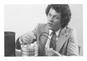
62. Cummins designed them with this keystone shape and exact 2° taper on the face to accurately maintain and control oil film on the liner wall.
