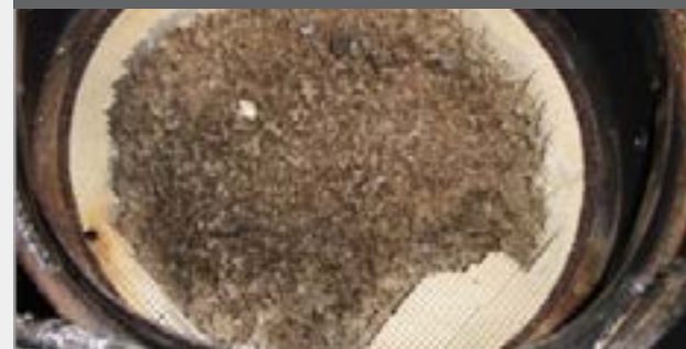
Cracked DPF Core
