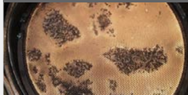
Melted DPF Core
