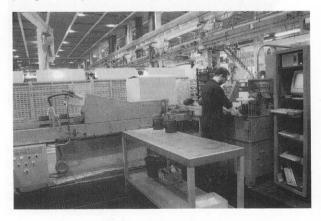
The machine compares each piston to a master sample and projects a separate ultrasonic signal from each piston location. Each piston is immersed in fluid to allow the signal to surround the piston surface. The acceptance/rejection is based on the signal seen by the PLC. Any failure data is stored and reported to Mahle on the monthly review process. The current capacity of the equipment is 400 pieces per day.
