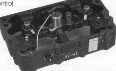
On the **air compressor**, the plumbing changes and the ring valve head design will improve efficiency. This will result in a higher output with a lower tank noise.
