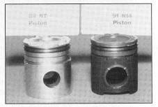
engines, such as the 460E. This is a surface treatment that increases surface/metal strength to resist cracking and gives the piston a dark gray color. This new piston is better able to resist cracking and corrosion and handle the higher temperatures encountered at the high torque output ratings of these engines. This anodized design increased piston cooling flow; thus, improving piston durability. The lower rated N14s will continue to use non-anodized pistons. The new piston also
