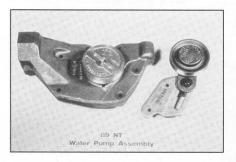
signed to include a new body casting, water pump impeller, beefed up bearing packs and idler, and increased grease flow capabilities. The water pump drive is similar to the BCIII inside idler with a poly vee six rib belt.
