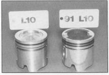
said before, the Ni-resist insert improves ring and ring groove life, giving your customers a longer life to overhaul. The top ring is specially lapped to hold extra oil to prevent scuffing and the crown of the piston is anodized to control the stresses of the higher cylinder pressures for a longer life to overhaul.
