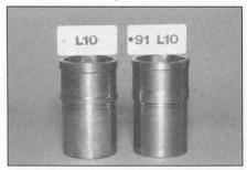
point on the outside of the liner as the top ring does on the inside. This keeps the rings cooler and reduces bore distortion for longer life and reduced oil consumption. The new liners **must not** be used in earlier style L10 blocks!
