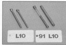
ing has increased in height and the rocker cover has been changed. Push tubes have replaced the original solid intake and exhaust valve push rods. The injector push rod is still solid. The push tubes and rods are 3/4 inch longer than before. The part numbers of the new intake and exhaust push tubes are identical, and are therefore interchangeable. More capscrew holes have been added to the rocker cover to improve loading on the gasket, making the joint highly resistant to leaks.
