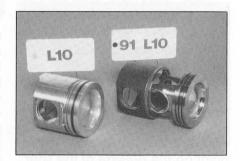
changes is in the piston. The L10 330E (330 horsepower with CELECT electronically controlled injection) has a new articulated piston. This piston has a forged steel crown and a separate aluminum skirt. The piston pin has been lengthened to accommodated the articulated piston design. The new pin is now 4mm longer for both the articulated pistons and the single-piece pistons for the lower horsepower L10s, a feature which makes the piston pin common between the two pistons.
